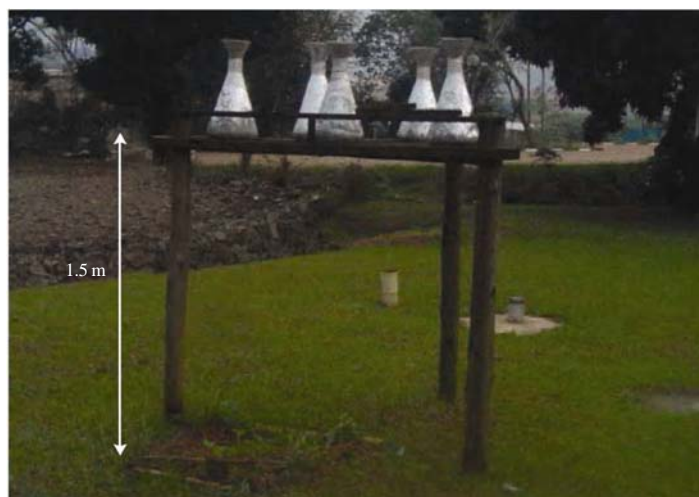
Fig. 2: Modified bulk sampler used in collection of rain water samples
