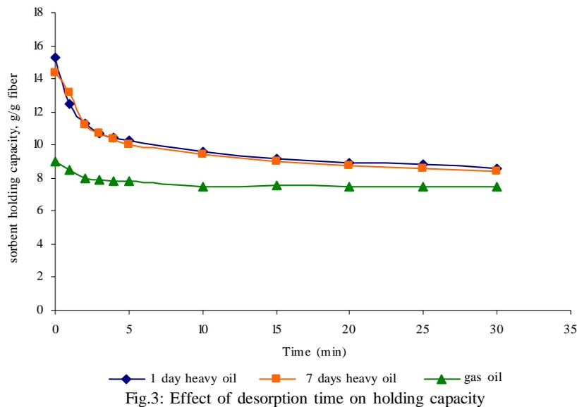
Fig.3: Effect of desorption time on holding capacity
