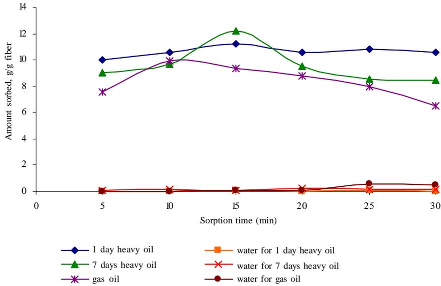
Fig. 2: Effect of sorption time on oil sorption capacity and water pick up
